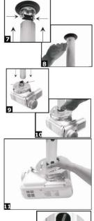
Join the extension tube to the ceiling by pressing the two spring loaded bolts on the ceiling plate in and by sliding the tube over, ensuring that the bolts click out of the holes accordingly.
