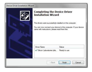
Step 5: Device Driver Installation Wizard found Silicon Laboratories Drivers. If not, the Drivers will be installed from internet. If the computer is not connected to internet, install Drivers from TB CD.
